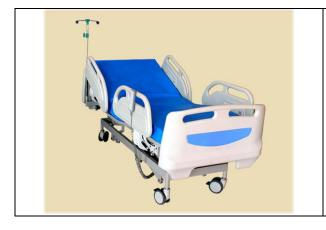
Specification: Frame work made of Rectangular M.S Tube MS Mattress platform in four sections Back Rest, Knee Rest, TB/RTB and Hi-Lo Positions obtained by electric actuator operator by hand remote system ABS molded head and foot bows ABS track away safety side Railing Telescopic IV Rod with Two Locations Chair / Flat Position Nurse Panel control Bed Mounted on 125 mm Dia Castor with central Braking system Overall Size: 210 L x 90W x 50 -70Hcms Finish: Epoxy Powder Coated
